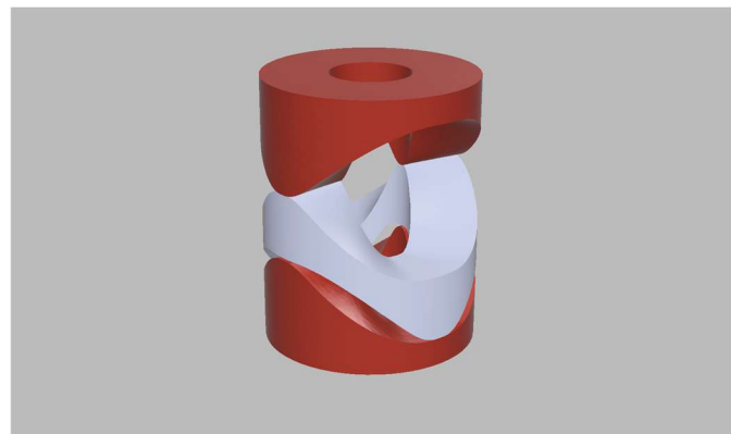
Figure 6. A real-world, annular implementation of the LESS mechanism, where the middle part (white) can rotate and reciprocate between the two external (red) stators.
