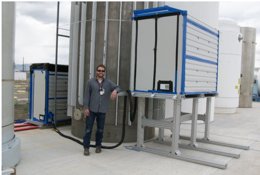
Fig. 29. Picture of the experimental setup with the two muon detectors on the opposite side of the cask. Source: Courtesy of C. Morris.
