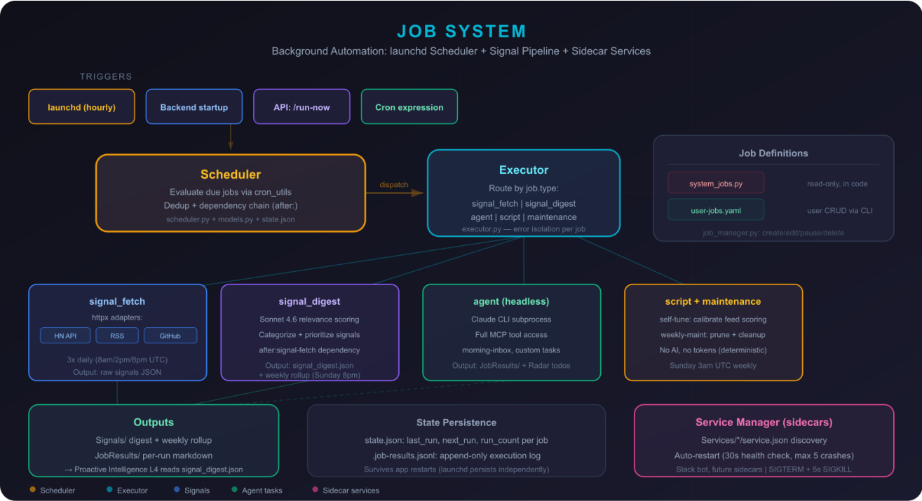
Figure 10: Job System — launchd scheduler, executor routing, signal pipeline, and sidecar services
